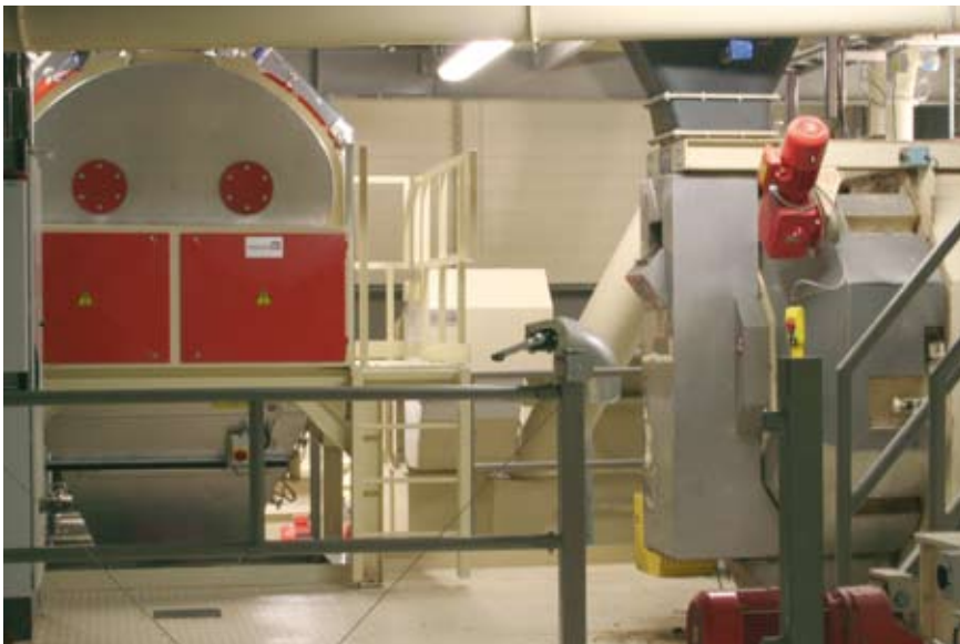
The Dinnissen vacuum coater is the core of the Magi-con feed manufacturing process
