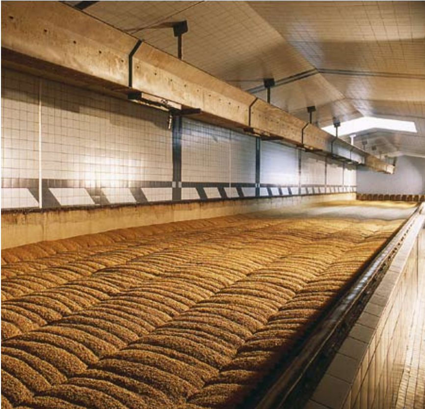
Large solid state fermentation unit at Soufflet's malting plant in Arcis-sur-Aube (Photo: Soufflet)
