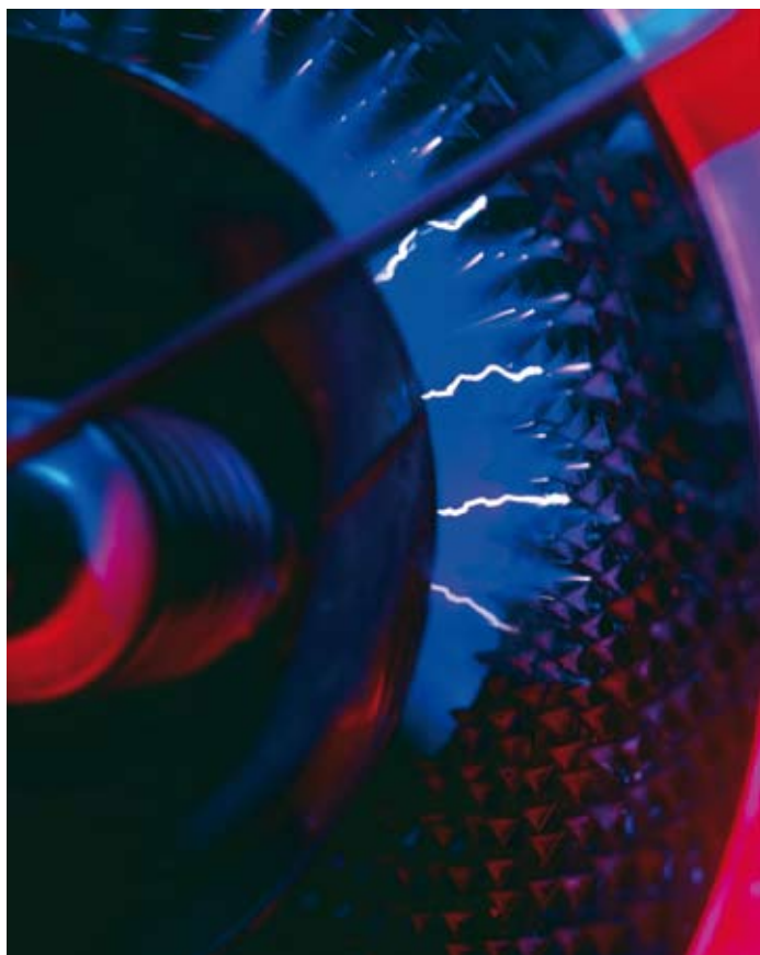
The blue colour is the Non-Thermal Plasma condition created inside the APP reactor
