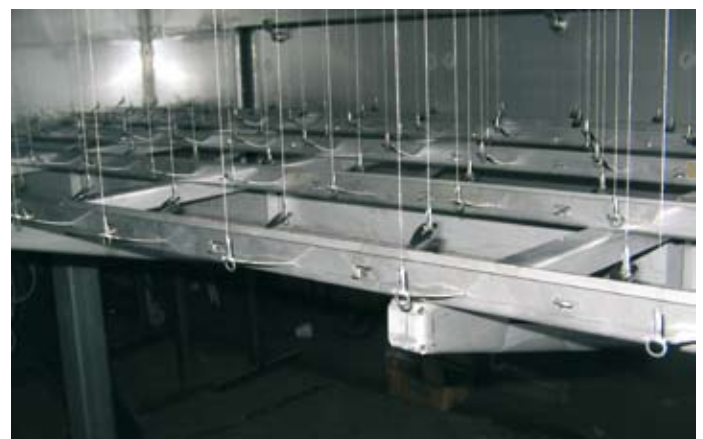
Lower electrode frame inside the reaction chamber
