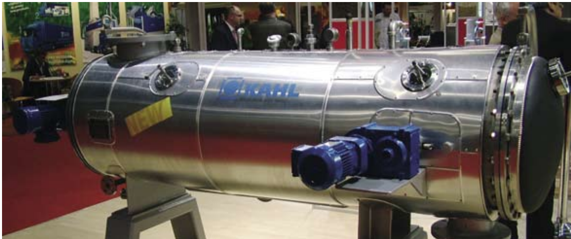
The new Kahl hydrothermal cooking plant is an alternative for a hygieniser, and is also capable of inactivating unwanted substances in raw materials.
