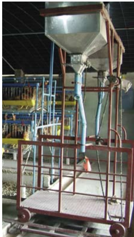
Feed is delivered to the hens by means of a home-made trolley with hopper and pipes to fill the troughs.
