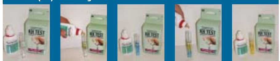
Figure 4 - A simple pond or aquarium water test kit determines the carbonate hardness (KH) of drinking water
