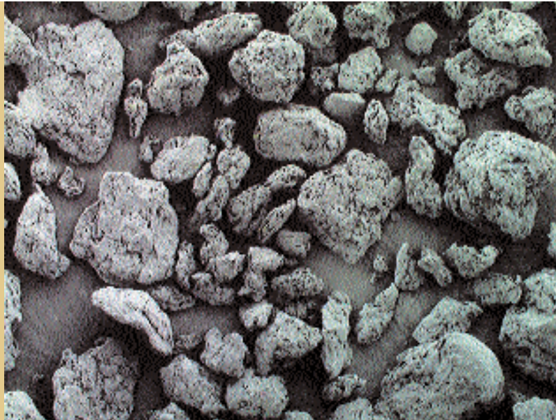
Photo 1 left - Electroscanning microscopial picture (62x) of a feed additive (generic diclazuril 0.5%) consisting of active material blend with a mineral carrier
