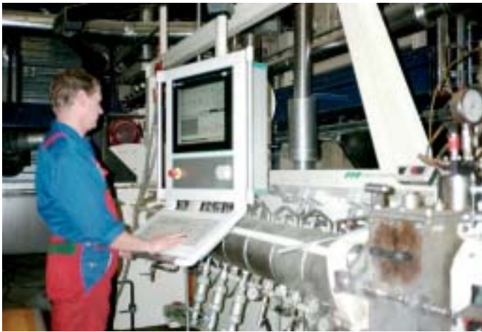
Extruder pilots can monitor the operation from their computers all the time, and any irregularities are revealed within 30 seconds.
