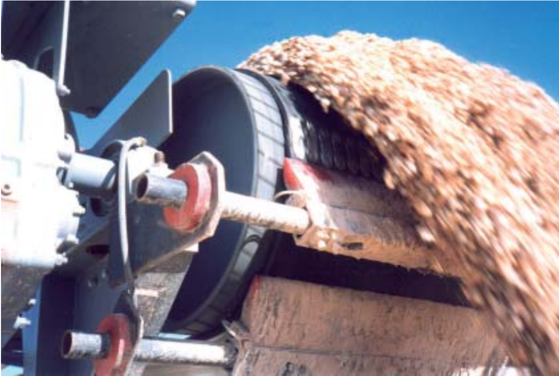
Belt cleaners have a positive effect on dust control by reducing carry-back that produces piles under the conveyor belt.
