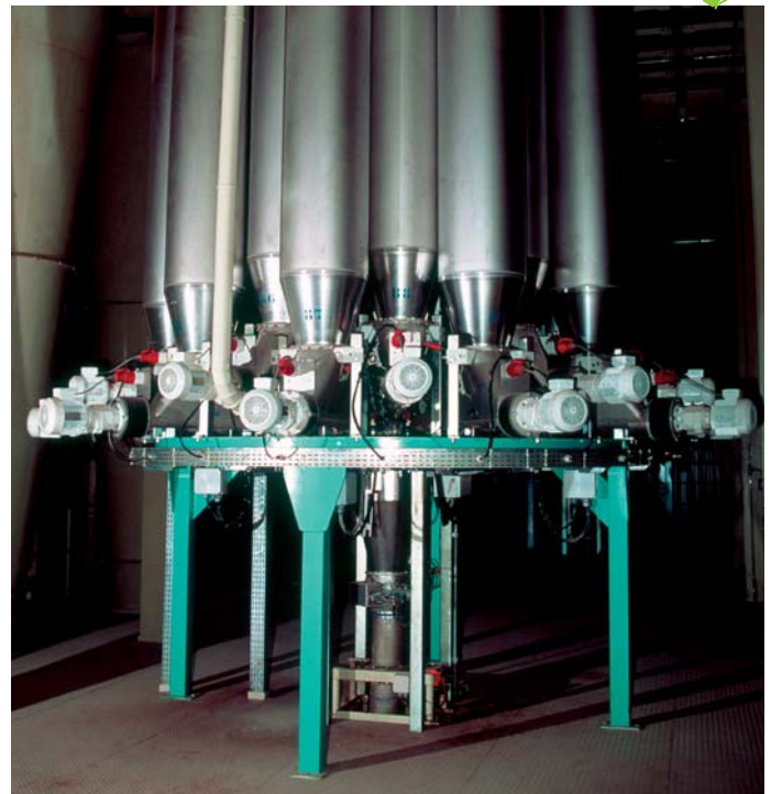
Micro proportioning unit: The micro-dosing unit has incorporated a scale of 50kg and is equipped with 20 silos (each 0.8 m 3 ) for the automatic addition of premixes to the main mixers.
