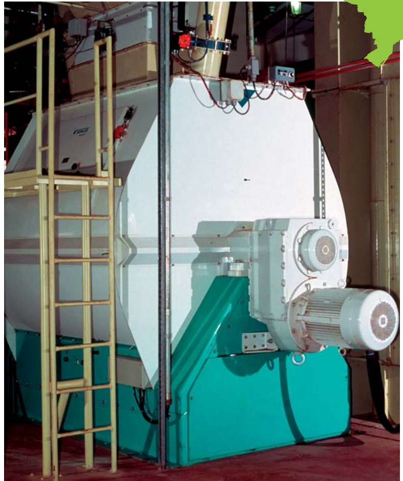
Main mixing: This is one of the main mixers with a usable volume of 8,000 litres and actual batch sizes of 5,000 kg, including liquid addition with swivel type spray bars and liquid scales for the preparation of the liquid mix.
