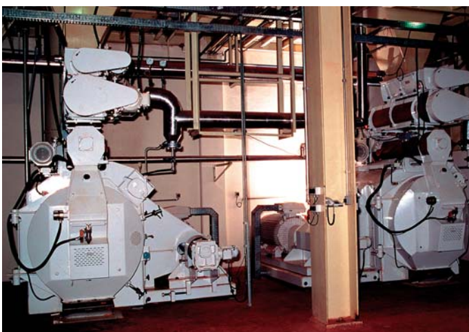
Pelleting: Four of these pelletmills are installed with a capacity of 30 t/h each, equipped with double conditioners including the surface heating system to reduce contamination and lower the bacteria count.
