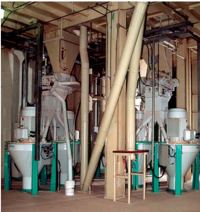
Grinding: Six vertical rotor mills, each equipped with a heavy particle separator and feeder, are divided into two groups to feed into the mixing lines. The set-up allows maintenance of each individual rotormill while all the others remain in operation.
