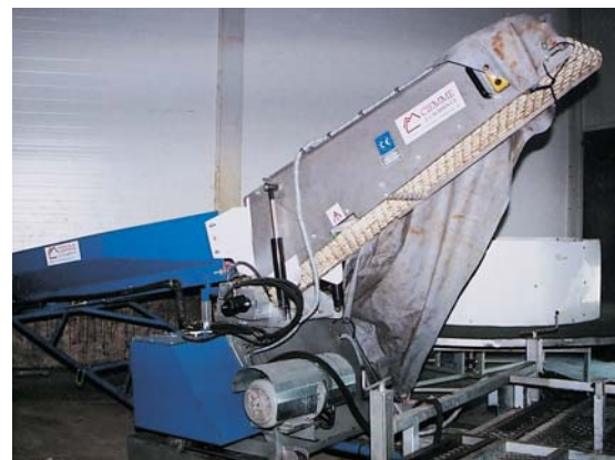
The transport belt delivers the birds to a Ciemme bird counter and crating machine, which delivers them semi-automatically into transport containers. There is no physical contact between the loaders and the birds at any time.
