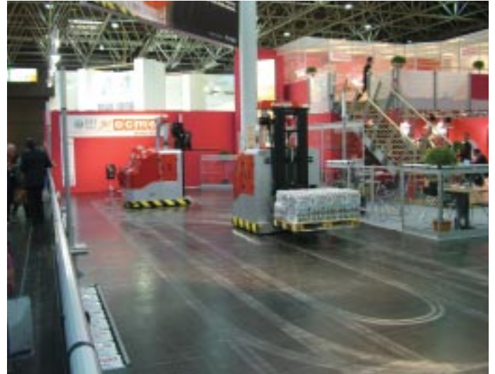
Laser guided vehicles can do the warehousing and have moved people to the control board. (Photo: Dick Ziggers)
