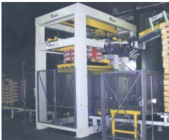
Modern palletising units can reach capacities of up to 1,200 bags per hour. (Photo: Newtec)
