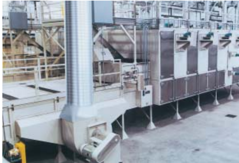
In pet food cooling and drying are combined and systems are large and very sophisticated. (Photo: ExtruTech)
