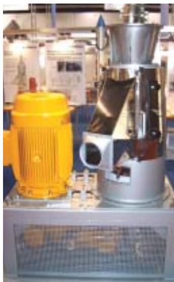
Kahl borrowed rice whitening techniques from sister company Schule to clean grain kernels of mycotoxins
