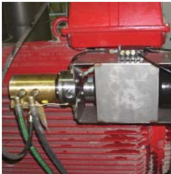
The hydraulic roll adjustment from Sprout Matador is placed outside the press chamber.
