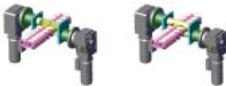
SME Control Module: Schematic of the valve rolls and actuators (extruder barrel not shown); Figure on left: closed position; Figure on right: open position
